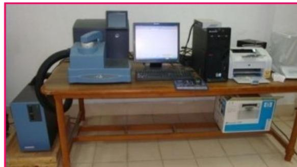
Fig.(4) Differential Scanning Calorimetry
